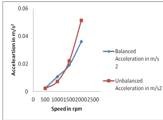
Figure4. Graph for comparison of balanced & unbalanced axial position
