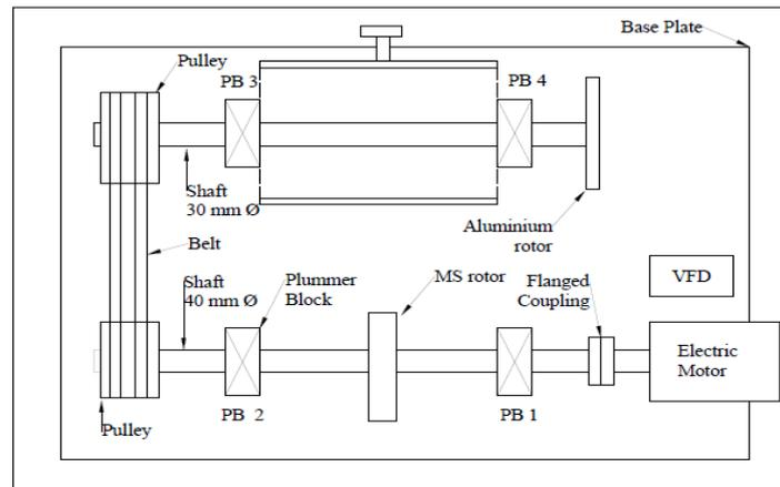
**Figure1.** Line diagram, top view of experimental setup
