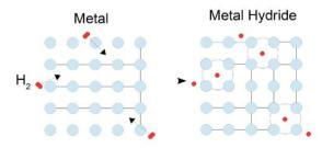
Figure 1. The basic principle of intermetallic hydrides [5]
