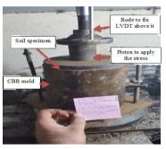
Figure6. Test setup
