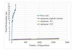
**Figure11.** Deformation of asphalt stabilized soil under Repeated loading in wheel tracking
