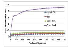
Figure 12. Deformation of asphalt stabilized soil under Repeated loading in PRLS
