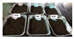
Figure3. Aeration of asphalt stabilized mixture
