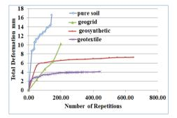
Figure9. Total deformation under wheel tracking test
