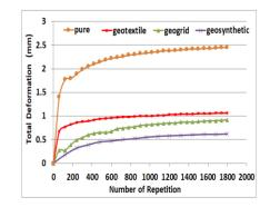
**Figure 10.** Total Deformation under Repeated loading in the PRLS
