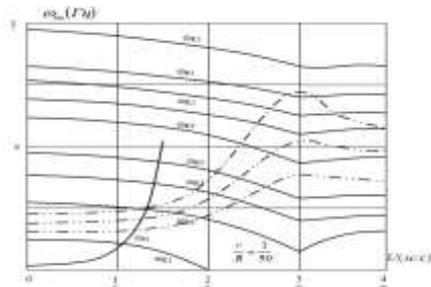
**Figure 7.** The change in the real parts of the natural frequencies of bending vibrations from the velocity of the flowing liquid.
