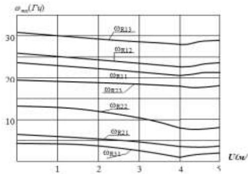
**Figure3.** The change in real parts of the natural frequencies of bending vibrations at different velocities of a flowing liquid  $h=0,005$ .
