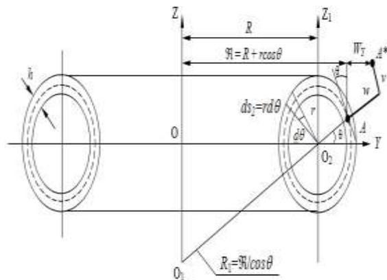
Figure 1. Curvilinear pipeline section in toroidal coordinates
