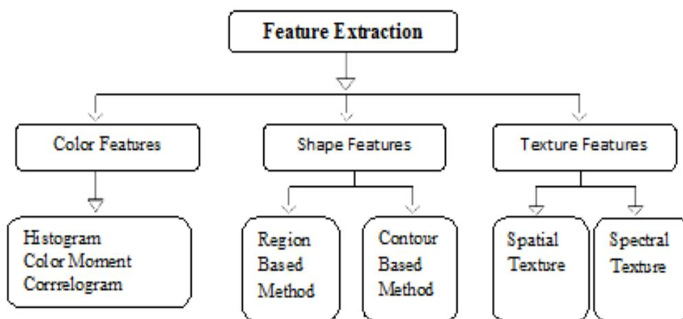
**Fig1.** Block Diagram of Feature Extraction
