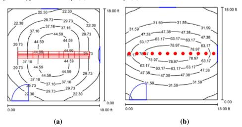
Line Arrangement of Fluorescent Lamps (A) And Led Lamps (B) Fig1. Average illuminance due to three arrangements of fluorescent and LED lamps in the room
