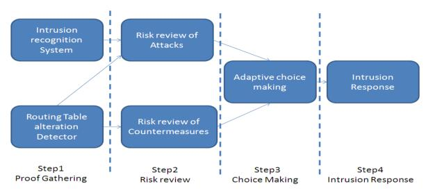
Fig1. Intrusion Response Mechanism for MANET routing attack
