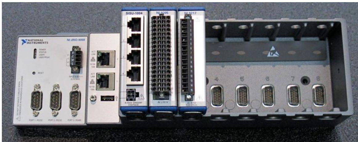
Figure2. NI RIO 9068 Real time FPGA control
